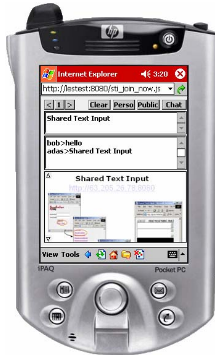
Figure 1. The Shared Text Input applet accessed from a PDA in Pocket Internet Explorer. Users can quickly type in notes by reusing words from the slide image (bottom) or from the notes taken by their friends (middle). Users simply tap the word they need to paste it into their notes.
