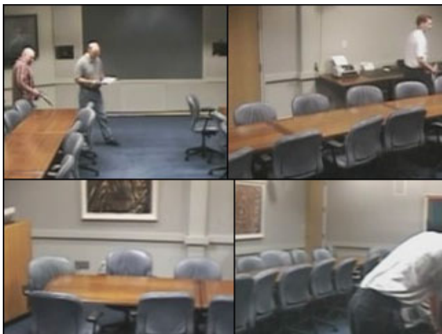
Figure 2. Quad representation of keyframes from four cameras with keyframes cropped to the center of activity and sized proportional to their importance.
