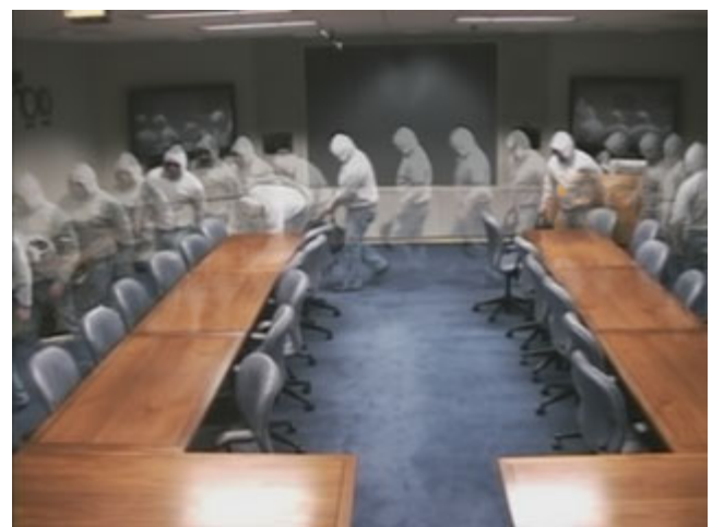
Figure 4. Alpha-blended foreground with 0.5 samples per second and more emphasis for every fourth sample.
