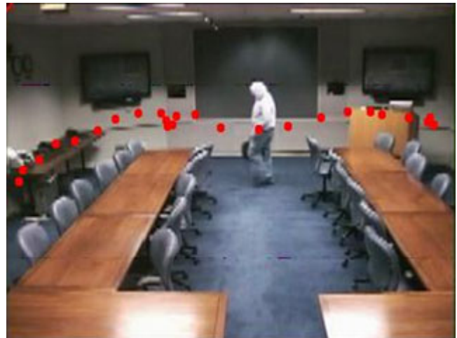
Figure 3. Trajectory of tracked object shown as dots marking positions at regular intervals.
