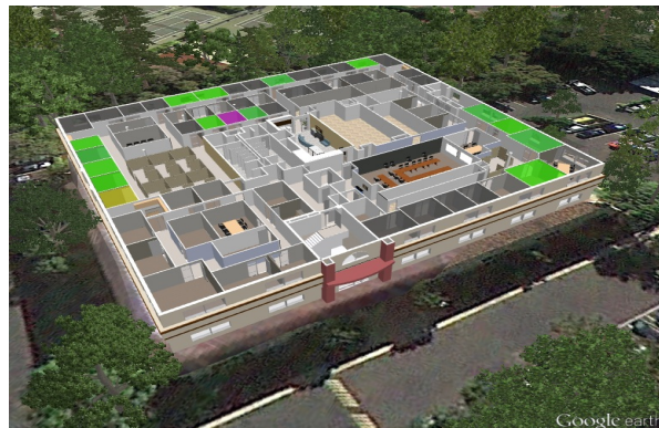
Fig. 1. Mirror world view of our Lab, shown in Google Earth. The color over a person’s office indicate whether that person is in the office (green), has a visitor (purple) or is in the building but out of office.
