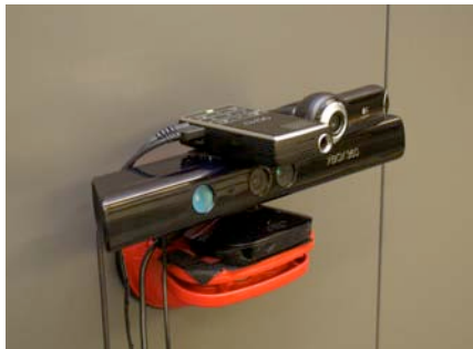
Figure 6. Hardware prototype using a Microsoft Kinect, mounted on a suction cup. The pico projector is placed on top of the Kinect. We have added a hi-res webcam on the right hand side.
