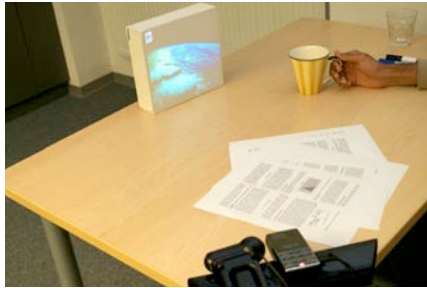
Figure 5. A photostream from Flickr is projected onto a box and can be navigated by rotating the coffee mug.
