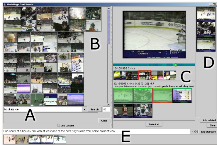
Fig. 4. The search interface. A text and image query is specified in area A. Query results are summarized as story keyframe collages in area B. Selecting a story expands the shots program timeline in area C. Relevant shots are collected in area D. the TRECVID topic is displayed in area E.
