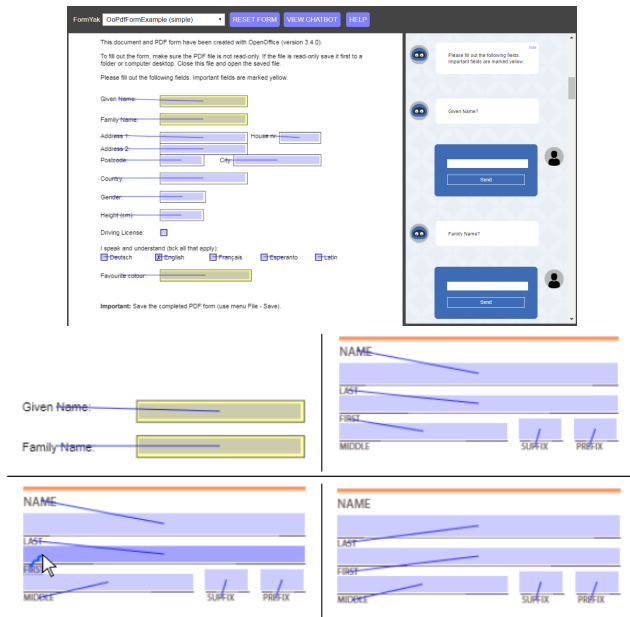
Figure 3: The FormYak web UI (top) attempts to associate all fields and labels. In some cases (middle left), it succeeds. However, in other cases (middle right) labels are assigned to incorrect fields. Users can draw a line connecting fields and labels to correct these errors (bottom).
