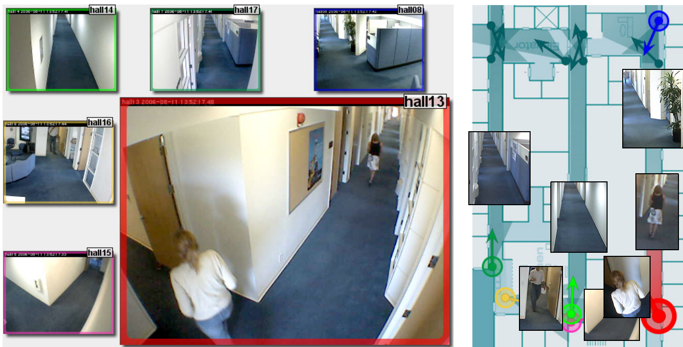
Figure 1. Video player surrounded by cameras in spatial proximity. The location of each smaller video approximately indicates the direction of that camera. The map on the right shows camera locations and parts of the camera views.
